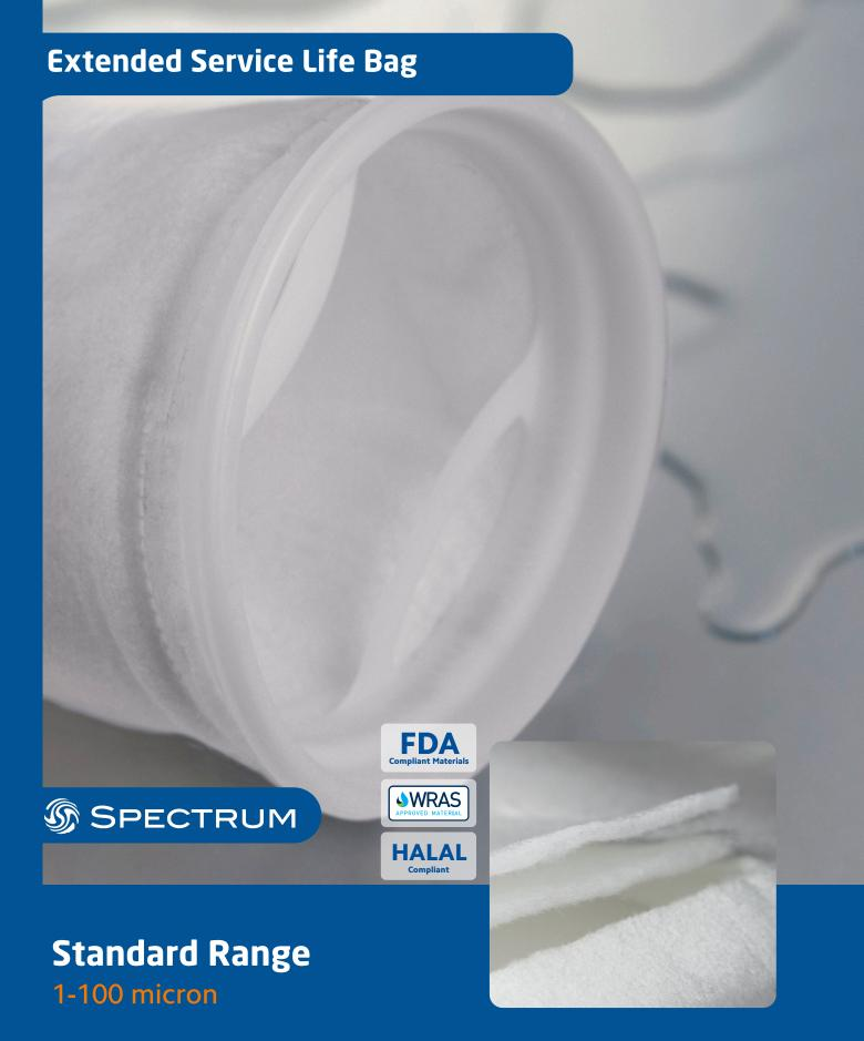
The Standard all welded construction of the SPECTRUM bag filter range prevents contamination bypass sometimes associated with stitching pin holes. Featuring a double-layer graded density construction, the first "pre-filter" layer traps larger particles and gelatinous contaminants, which often cause premature blinding, with the second, finer filtration layer effectively trapping unwanted particulate.
